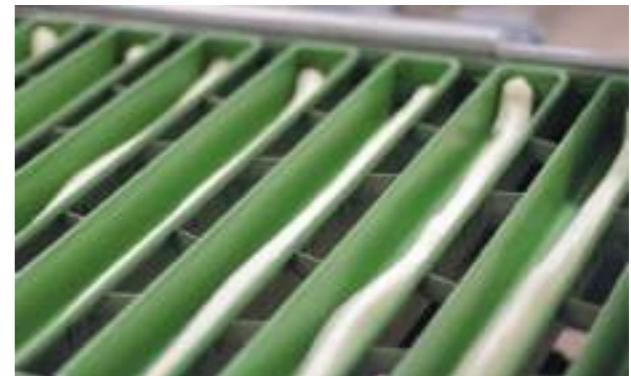
The dough is divided into uniform portions that are worked to obtain the ideal shape to be automatically placed inside the molds.
