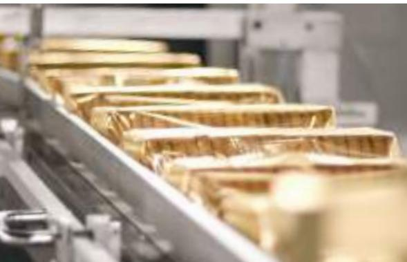
Leaving the oven, the toasts are properly grouped and wrapped with film. Each package is placed in transport boxes, waiting in the logistic warehouse for shipment to one of our customers somewhere around the world.
